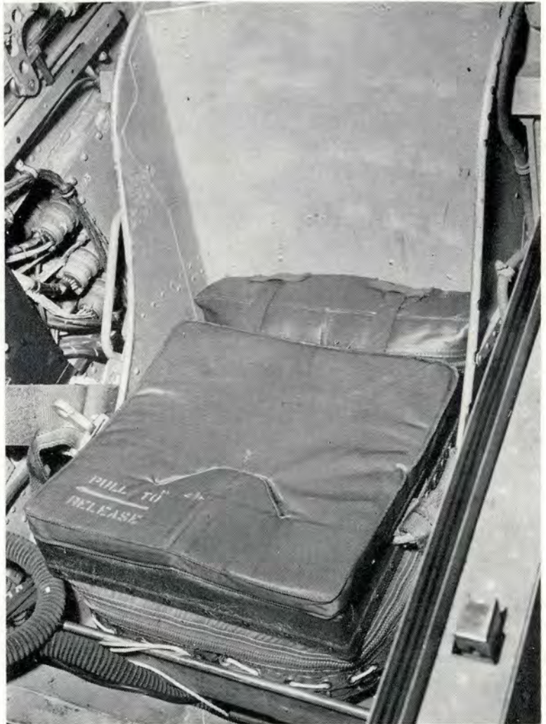
Upper photo shows sleeping bag in stowed position. Illustration below gives top view of pack and attachment straps.
